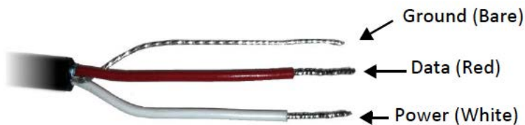
Figure 2: Pigtail End Wiring
