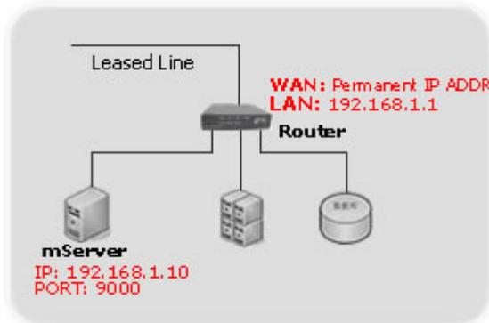
The mServer's IP address for the remote MD-609G is the IP address of the router's WAN interface. Please check the status information on the router of go to <http://www.ip138.com>.
