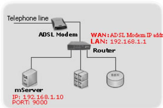
The IP address to be configured in MD-609G is the same as the IP address of the router's WAN interface. The IP address can be obtained through the website <http://www.ip138.com> or by checking the status information on the router.
