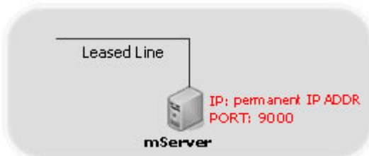
The IP address of mServer is a public address, and it can be checked by using the "IPconfig" command or going to the website <http://www.ip138.com>.
