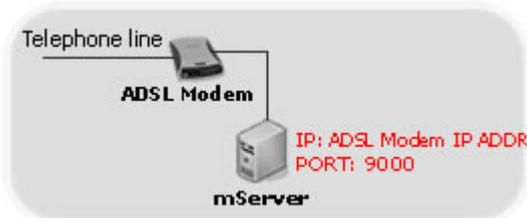
The IP address to be configured in MD-609G is the IP address of the computer. The IP address can be obtained by using "ipconfig" command or through the website <http://www.ip138.com>.
