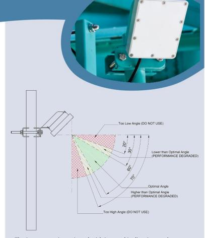
The instrument is equipped with internal inclination angle sensor. The measured inclination (tilt angle) is reported by the instrument and can be seen in the PC application for instrument configuration. It is strongly recommended to check the inclination measured by the instrument itself during equipment installation. This measurement is also used internally for automatic velocity cosine compensation.
