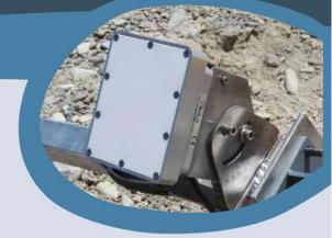
In both directions, so for such sites, the radar sensor should be configured to report both incoming and outgoing flow, by selecting "both direction" setting in the radar sensor.
