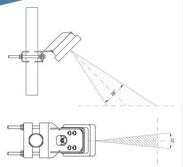
The water flow at the installation site should be as uniform as possible. Reliable measurements will be obtained if the river channel is straight for at least 100 meters before the site, without curves and changes in the channel width. The water should be free from any turbulences such as vortexes, and should be at least 100 meters away from weirs or waterfalls.
